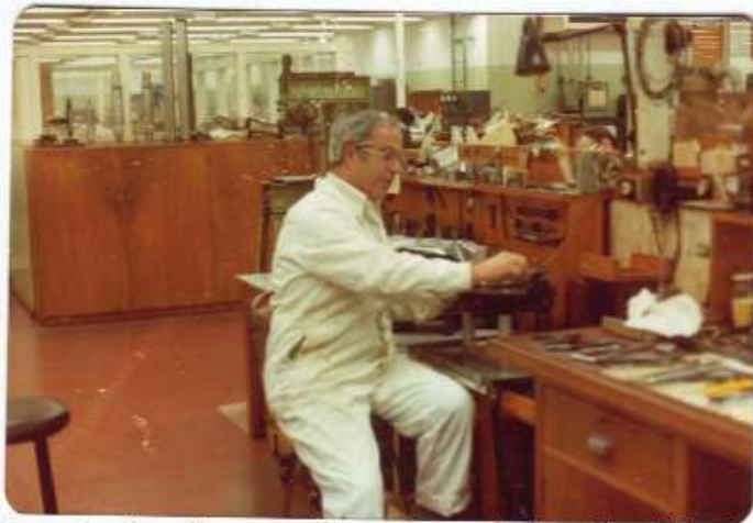
Here is the disassembly and repair bench of the constant speed drives .
